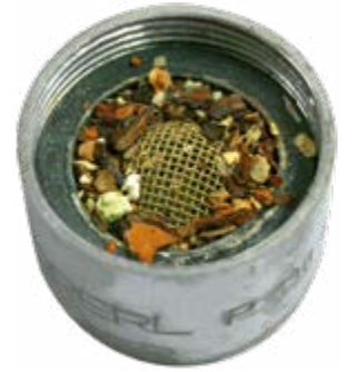
Rust particles in a tap sieve indicate corrosion is present
